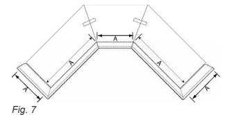
2. Mark your first measurement, for example, begin left to right in installation of Fig. 7, using the shelf depth as your first cut to mark. From the 90° end cut of the panel, mark the distance 14" in the groove on the back of the molding (Fig. 8). (The groove is aligned directly over the front edge of the top of the cabinet.)
